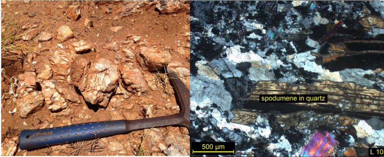
**Figure 1:** Spodumene crystal in the weathered discovery pegmatite and petrography
